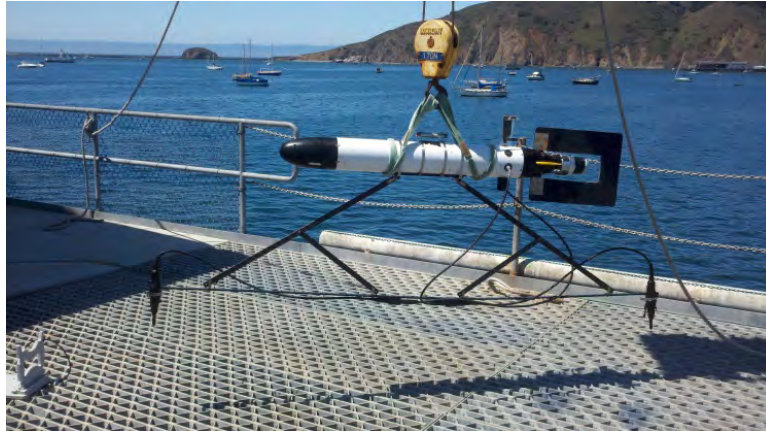
Figure 2.14: The Rig Used to Fix the Hydrophones under the AUV
