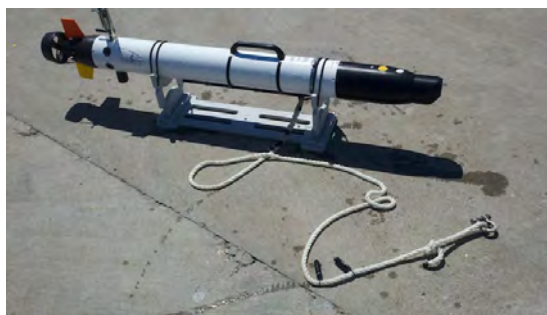
Figure 4.3: Transmitter Attached to The Second AUV
