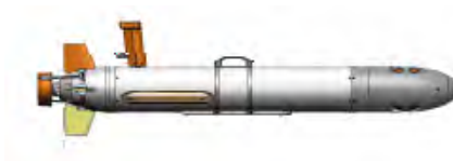
Figure 2.8: Autonomous Underwater Vehicle Used in the Current Research
