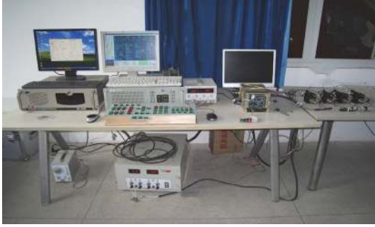
FIGURE 10: Hardware in the loop simulation platform.
