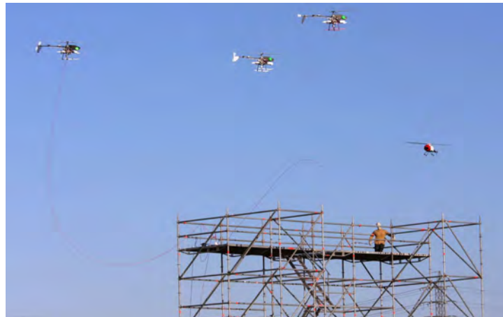
Figure 15: Three UAVs transporting a pan-tilt wireless camera to the roof of a building with a height of 12 meters in Utrera (Spain) in May 2009. The images show the mission during the take off (topmost picture), during the actual load transportation (middle-left picture), shortly before (middle-right picture) and shortly after the load deployment (bottommost picture). On two pictures a fourth helicopter is visible, which was used to acquire airborne video footage of the mission.
