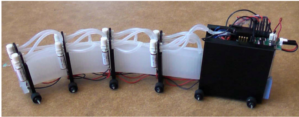
Figure 1. Experimental prototype of the fluidic elastomer robotic snake. The body consists of four bidirectional fluidic elastomer actuators in series. Valves and passive wheels are attached between segments. The electronics and energy supply are inside the tail on the right.
