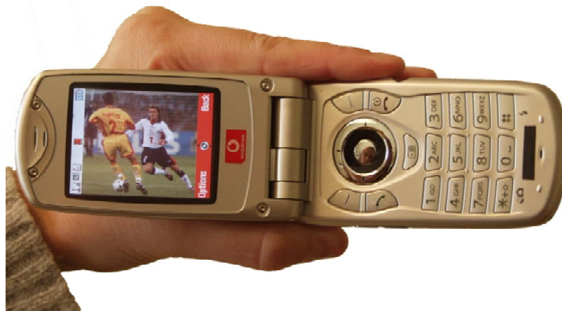
Fig.8 Handset with Ocuity Polarisation Activated Microlens and Swedish LCD Centre plastic LCD
