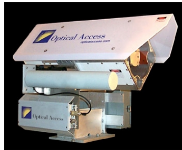
Figure 5 A FSO terminal with RF back-up. The multiple transmitters and larger receive aperture of the FSO terminal are features which reduce atmospheric scintillation. 8 The radio back-up can increase the availability of the hybrid wireless system to 99.999% at long ranges (see Figure 7).
