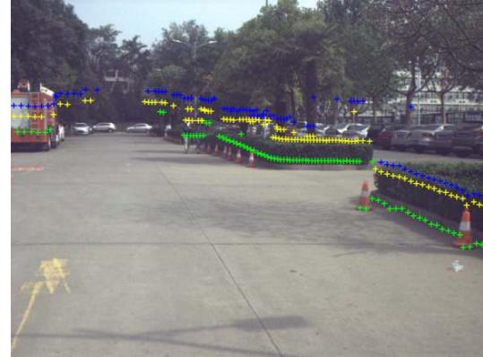
Fig. 12 A scenario in which the pedestrian in the front was discarded incorrectly because the road is uphill, which causes an incorrect mapping of LIDAR data to the image (References to color refer to the online version of this figure)
