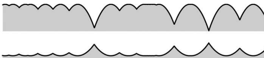
Figure A5. Cross-section of heights for the surface in the middle row of Figure A4. The top profile shows a sample of the surface itself, the bottom row a sample of a depth-inverted version. The two types are easy enough to distinguish; thus, you can easily notice whether you see the surface (or perhaps only part of the surface) in the images of the middle row of Figure A4 as intended, or reversed. You may want to practice on the leftmost image. You should be able to “get” (in visual awareness) both the correct and the inverted version. In the rightmost image, you may notice correct and inverted patches, shifting as you change your fixation.
