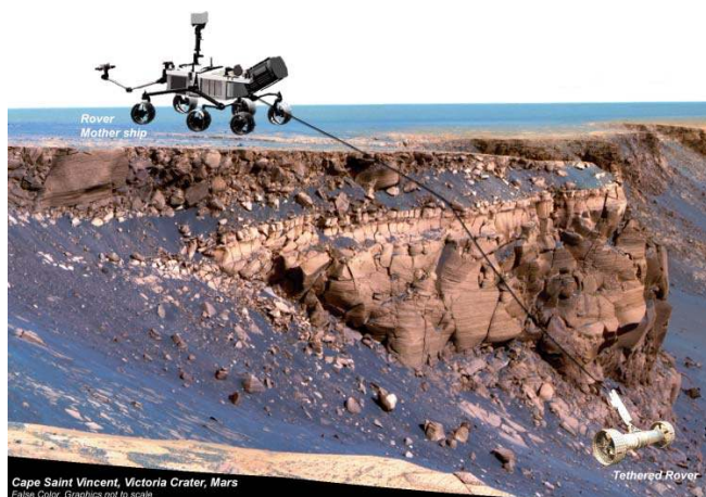
Fig. 3. Proposed mission concept overlaid on false color image of Victoria Crater. Note that the rover graphics are not to scale.
