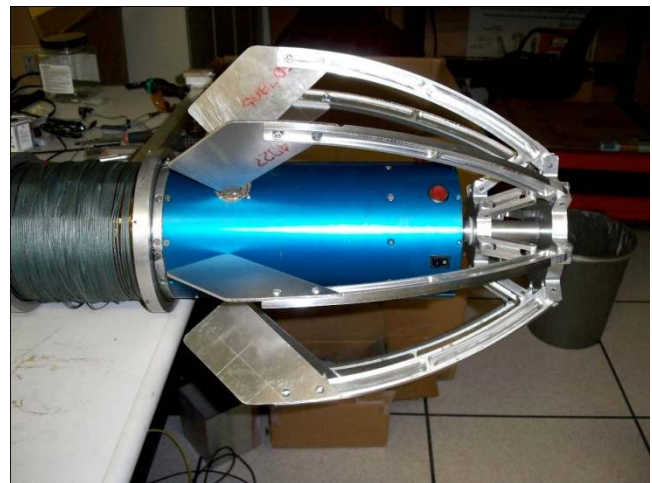
Fig. 10. Unfolding wheel prototype collapsed around Axel. Secondary plate can be seen just adjacent to the rover's body.
