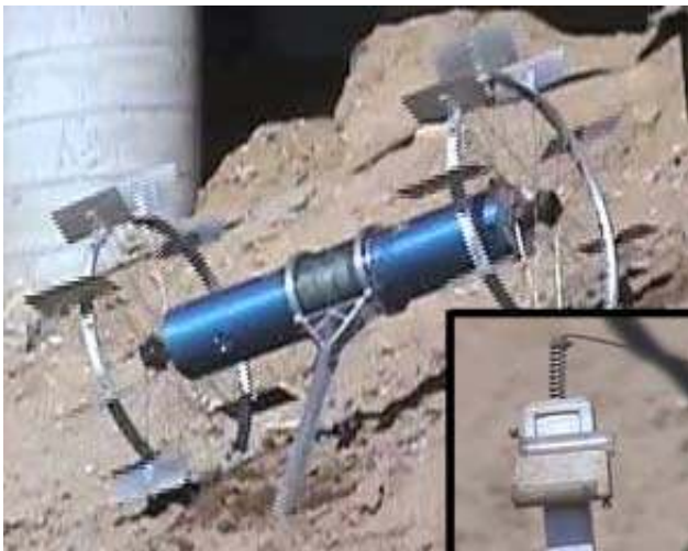
Fig. 4. Axel taking a sample by pointing the caster arm into the ground and turning in place. Sand enters through the openings on the ends of the removable sampling tubes (inset).
