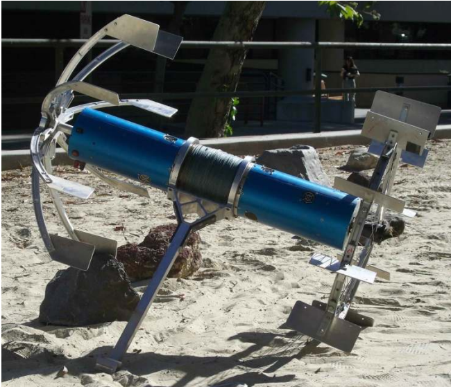
Fig. 11. Unfolding wheel prototype in expanded state mounted alongside original paddle wheel. The wheel is travelling over a rock approximately 1/3 of its diameter.
