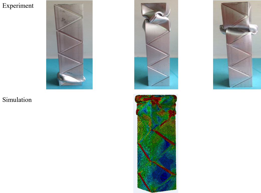
Figure 19. Failure modes from experiment and simulation for axial impact loading
