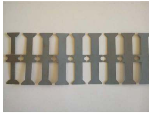
Fig. 10. Serpentine cut out of the soft magnetic material. The laminations are connected in the middle through little joints. Subsequently, the serpentine is folded into a stator-core element.
