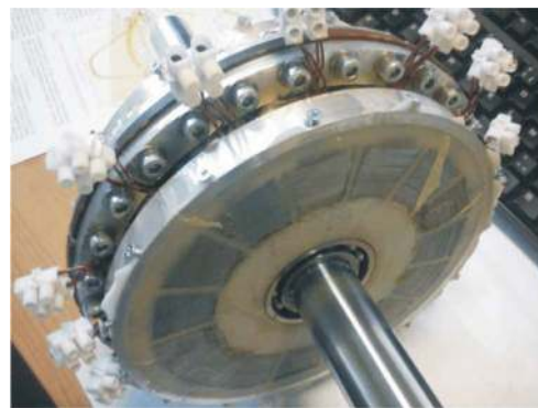
Fig. 11. Finished stator consisting of 15 pre-made stator-core elements. Axial positioning and fixation of the elements is achieved at the middle of the stator cores.
