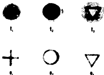
Fig. 10. Tomograms ( t_1, t_2, t_3 ) and their reconstructions ( o_1, o_2, o_3 ) using a wire proportional chamber and the pinhole array of Fig. 2a.
