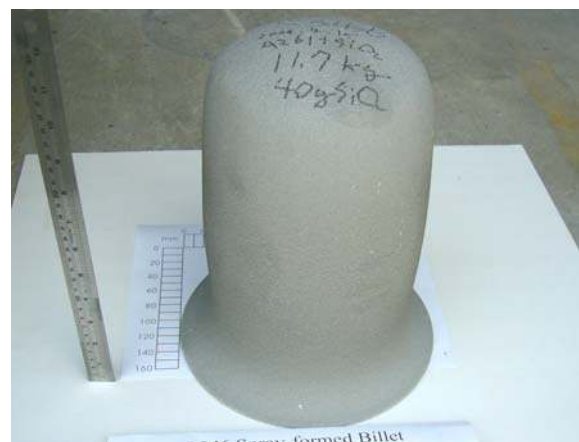
Fig. 4 Photograph of a successful spray formed Mg/ \text{SiO}_2 composite billet.
