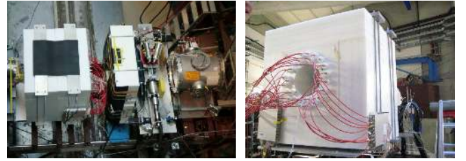
FIG. 7. Left: Top view of BELEN and the front PE-shielding wall (beam enters from the right-hand side). Right: Picture of the BELEN detector showing the two rings of counters, the central hole where SIMBA (see Fig. 3) was placed and the extra 20 cm of PE shielding around.
