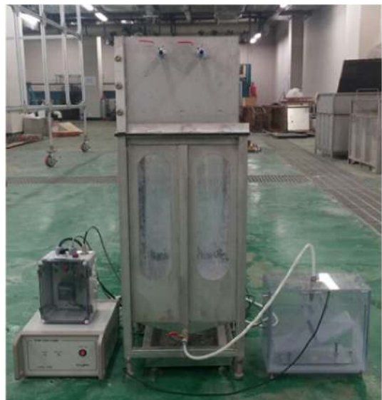
Fig. 4. Infiltrometer for permeable pavement systems.
