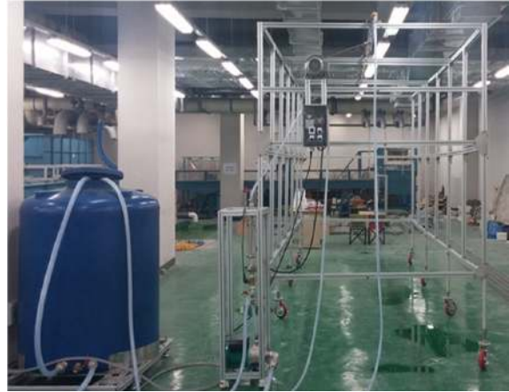
Fig. 3. Mobile rainfall simulator.
