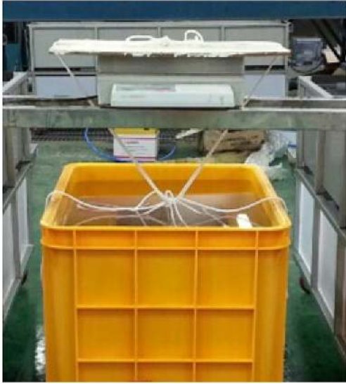
Fig. 2. Equipment to measure submerged weight.
