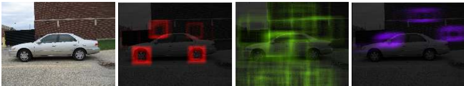
Figure 3: Part detector responses for left front wheel (red), left front door (green), and windshield (magenta), overlaid onto the original image (left). For each part, we show an accumulation of bounding boxes, weighted by detector response, drawn at the respective location and scale.
