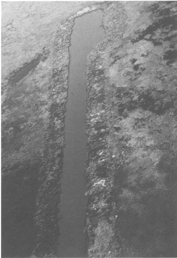
Figure 4. No emergent marsh was established in the Buckskin Bayou backfilled canal despite the use of most available spoil material as fill.
