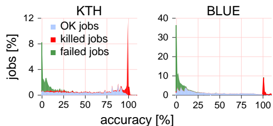
Figure 2: The accuracy histogram is rather flat when ignoring jobs that reached their estimate and were killed by the system (100% peak) or that failed on startup (0% hump).
