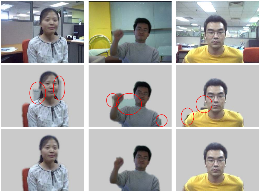
Fig. 7. Comparison with the basic model. Top row: a frame in a video sequence. Second row: result by the basic model. Red circles indicate notable segmentation errors. Last row: result by background cut.
