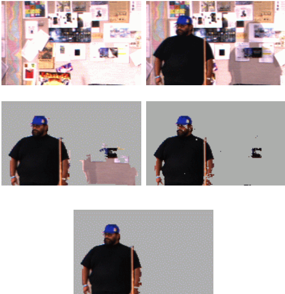
Figure 4. Top: Background image, person in foreground casting a strong shadow. Middle left: Basic color segmentation, shadow remains. Middle right: Effect on color segmentation when using the higher threshold for the entire image: skin tones close to background color are eroded. Bottom: large portions of shadow removed with adaptive (range-based) threshold.
