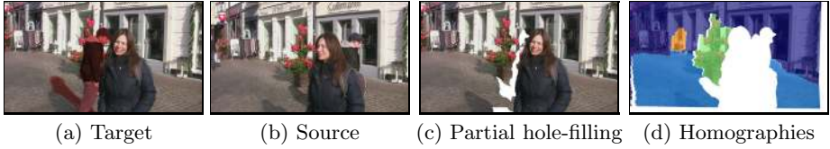
Fig. 2. Homography-based alignment. (a) Target frame with the region to be inpainted shaded in red; (b) a source frame where the region to be inpainted is partially visible; (c) target frame partially filled using the aligned source; (d) overlay between the aligned source and the mapping K that selects the homography used to align each region.
