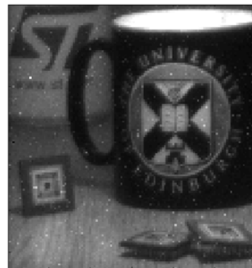
Fig. 3. Single shot grayscale intensity image with no post processing. White dots are high DCR pixels.
