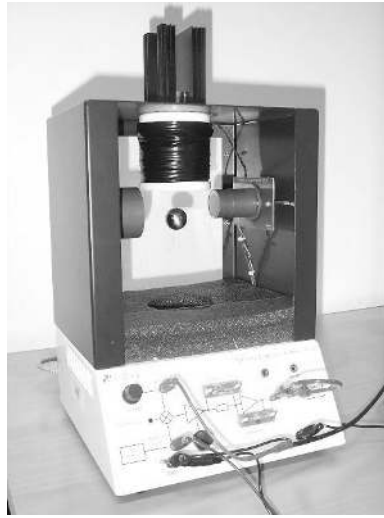
Figure 6.4: A magnetic levitation system in which an electromagnet is used to make a steel ball levitate.
