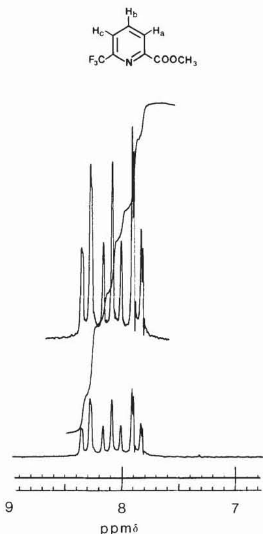
Fig. 3. ^1\text{H-NMR} spectrum of methylester of 6-TFM-2-picolinic acid, a derivative of metabolite M2. The 100-MHz-spectrum of the compound in deuterated chloroform was recorded with tetramethylsilane (TMS) as internal standard
