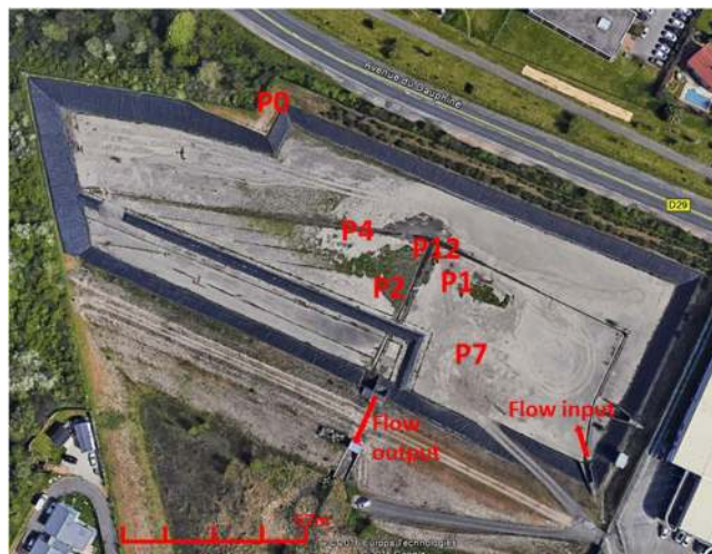
Figure 1. Numbered position of each sampling site (P) of the Django Reinhardt detention basin (DjR DB) of the “mi-plaine” industrial zone of Chassieu (France). Red arrows indicate the runoff entry point, and outflow of the detention basin. The outflow is directed toward an infiltration basin connected to the Lyon east aquifer. P0 was the control site located outside but at the edge of the detention basin. P12 is a decantation pit. Recent deposits can be observed in the DB.
