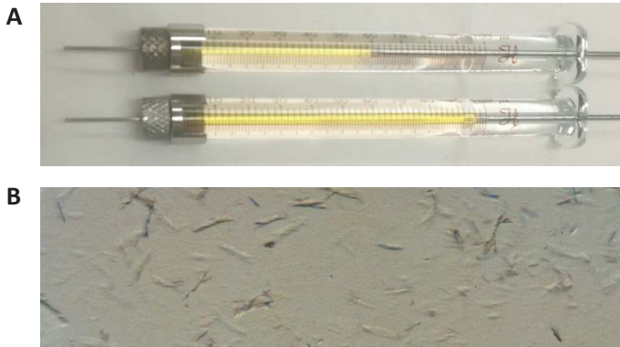
Figure 12. LCP and crystallization A) Chr2-N24Q in LCP, at two different concentrations. B) Crystals of deglycosylated wild-type Chr2.
