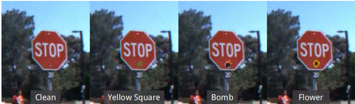
FIGURE 7. A stop sign from the U.S. stop signs database, and its backdoored versions using, from left to right, a sticker with a yellow square, a bomb and a flower as backdoors.
