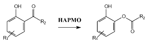
Scheme 3. Biocatalytic production of protected catechols using HAPMO.
