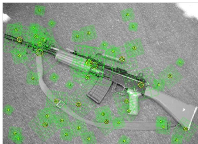
Figure 2. Showing a Selected 50 out of 17251 SIFT Descriptors Displayed on a Fire Weapon
