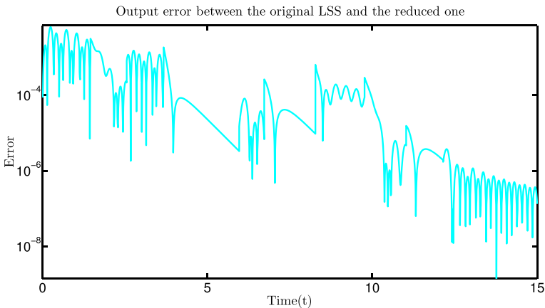
Fig. 2 Absolute value of the output error: |\mathbf{y} - \hat{\mathbf{y}}|
