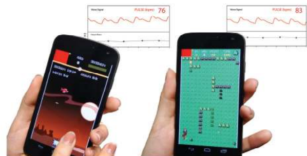
Figure 1. Real-time heart rate measurement via LivePulse Games (left: City Defender, right: Gold Miner).
