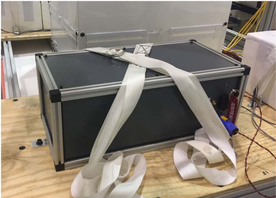
Fig. 5 GMoDem bolted and strapped to the ASCOT gondola
