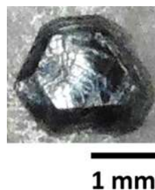
FIG. 4. Appearance of an as-synthesized w -BN crystal. Reproduced with permission from Deura et al. , Jpn. J. Appl. Phys., Part I 56 , 030301 (2017). Copyright 2017 The Japan Society of Applied Physics.
