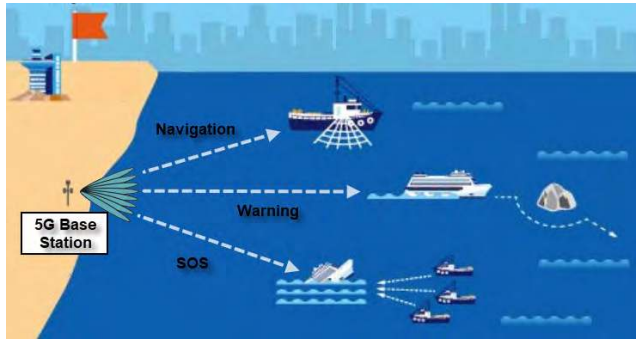
FIGURE 1. Illustration of 1-D beam steering in the horizontal plane required in based stations for offshore maritime communications.
