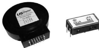
Fig. 1. US Digital inclinometer (left), Murata gyroscope (right). For scale, note that the connection wires are 0.1 inch apart.
