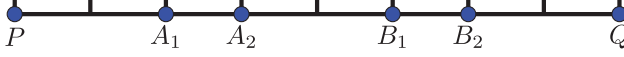
Fig. 5. The sensors' locations: x_P = 0; x_{A_1} = \frac{1}{4}S_1; x_{A_2} = \frac{3}{8}S_1; x_{B_1} = \frac{5}{8}S_1; x_{B_2} = \frac{3}{4}S_1; x_Q = S_1 .
