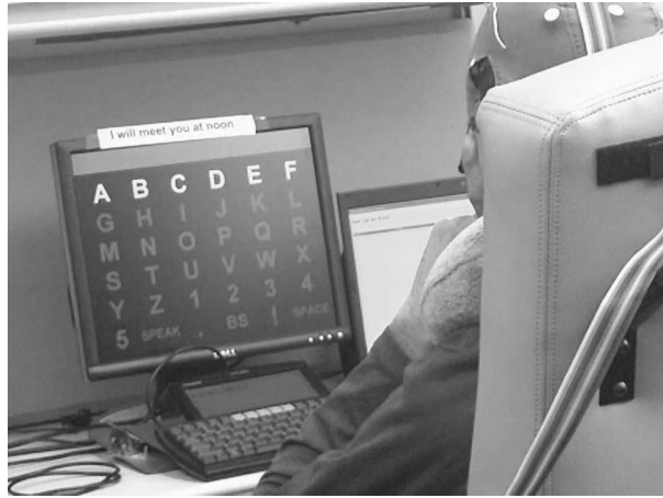
Figure 1. The setup of the P300-based BCI experienced by focus group participants with ALS. Individuals sat in front of a computer screen which displayed a 6 \times 6 grid of letters and commands; rows and columns of the grid flashed in a seemingly random manner. Brain activity was recorded from the EEG cap donned by the BCI user.
