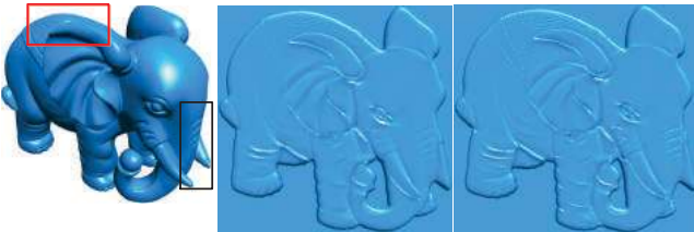
Fig. 25. Bas-relief modeling on elephant. From the left column to the right: The input model, the results Schuller et al. [20], and our detail-enhancement results ( \mu = 0.3, \beta = 0.2, \delta = 10 ).
