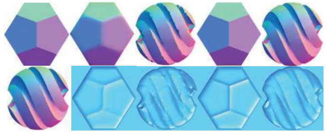
Fig. 6. Using RNF plus GMM can prevent shape distortion of the base surface. The first row shows the original normal map (the first one), the base normal maps obtained by the RNF (the second two) and the GRNF (the last two) respectively; the second row shows the original normal map (the first one) and the bas-relief modeling results from their upper counterparts. Compared to the results by the RNF, the results by the GRNF can better preserve the base’s structures.
