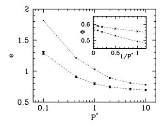
FIG. 7. Main plot: void ratios in primary isotropic compression,  $e_{iso}$  (square dots), and in critical state,  $e_0$  (crosses with error bars) versus  $\log P^*$ . Inset: detail of variations of solid fraction  $\Phi_{iso}$  in isotropic compression (square dots), and  $\Phi_0$ , in critical state (crosses), for large  $P^*$  (including the dry case of infinite  $P^*$ ), versus  $1/P^*$ . Dashed lines are drawn to guide the eye.
