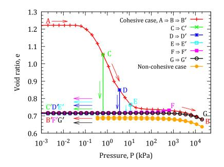
FIG. 5. Void ratio versus reduced pressure  $P^*$ , as cohesive forces are suppressed at the beginning of unloading, starting at different points on the primary compression curve. (In this case the initial state had solid fraction  $\Phi_0 = 0.45$ ).
