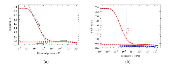
FIG. 2. (a) Effect of cycle of pressure (in dimensionless form) on void ratio. The straight line fits the curve for intermediate  $P^*$  values. (b) Same curve, compared to result obtained with dry, cohesionless grains (bottom curve, crosses joined by dark line), with pressure in kPa, for glass beads with a = 0.115 mm, wet by water.
