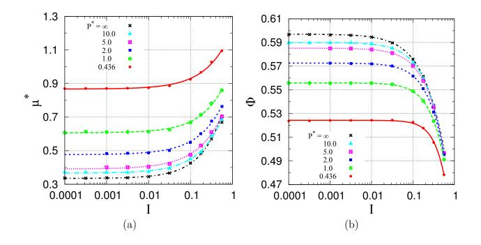
FIG. 6. (a) Internal friction coefficient  $\mu^*$  and (b) solid fraction  $\Phi$  versus I for different values of  $P^*$ .
