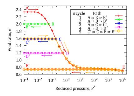
FIG. 3. Effect of different (isotropic) unloading and reloading histories on void ratio. The system does not rearrange along unloading paths BB', CC', DD', EE', which are reversible. Path 5 causes plastic response in section CE, along which pressure increases beyond its past maximum. The primary curve (path 4) is then retraced.
