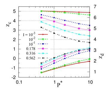
FIG. 8. Coordination numbers of contacts  $z_c$  (left axis, upper curves) and of distant interactions  $z_d$  (right axis, bottom curves), versus reduced pressure for different values of I.
