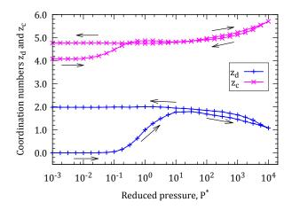
FIG. 4. Evolution of coordination numbers of contacts  $z_c$  and of distant interactions  $z_d$ , in the pressure cycle of Fig. 2(a).
