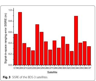
Figure 3 shows that the average SISRE is approximately 0.474 m, and all the SISREs are in agreement with the satellite clock offsets. The SISRE of the M02, M06 and M15 satellites are significantly greater than those of other satellites; when BDS-3 started offering global service in December 2018, the SISRE was approximately 0.7 m.
