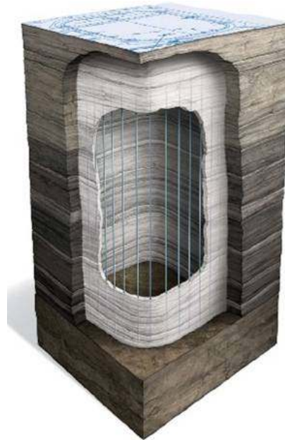
Figure 1. Schematic of Shell ICP process using freeze wall technology for producing fuel from oil shale.
