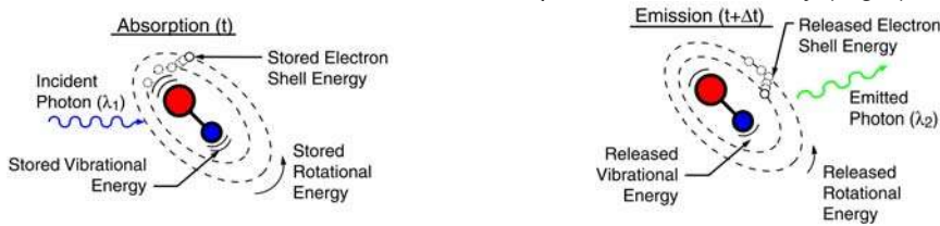
Figure 1: Schematic illustration of laser induced fluorescence. A photon of wavelength (color) \lambda_1 excites an electron to a higher energy state. When the electron returns to its original state it emits light of wavelength \lambda_2 . The emission intensity is linked to temperature and concentration of the molecules. The color of the absorbed and emitted light is specific for each type of molecule, thus finger-printing at a molecular level is enabled.
