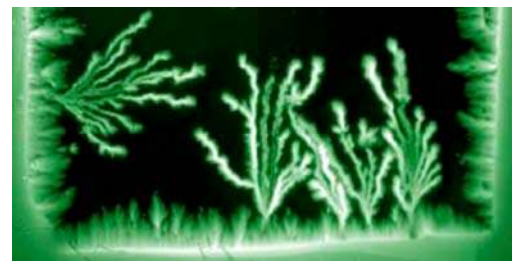
Figure 32 Magneto-optical image of magnetic flux avalanches penetrating into a \text{MgB}_2 film at 5 K (Image courtesy of T.H. Johansen, University of Oslo).
