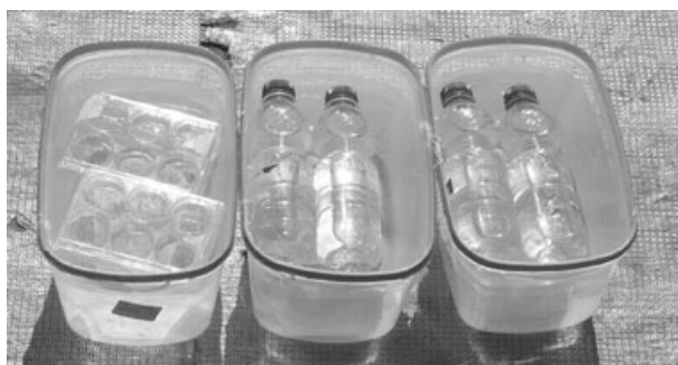
Figure 2 Escherichia coli suspensions contained in transparent polystyrene six-well plates (on the left) and polyethylene terephthalate 300-ml bottles (centre and right) immersed in 3 l water baths, and exposed to strong natural sunlight on the laboratory roof in Southern Spain.
