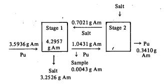
From this material balance, the fractions of americium partitioning to the salt  $(f_s)$  and metal  $(f_m)$ were obtained for each stage and for the overall extraction. The fraction of americium partitioning to the metal  $(f_m)$  was used to determine the values of the extraction factors (a) obtained in each stage and in the overall extraction. The values were calculated using Equations 3 and 7, respectively.
