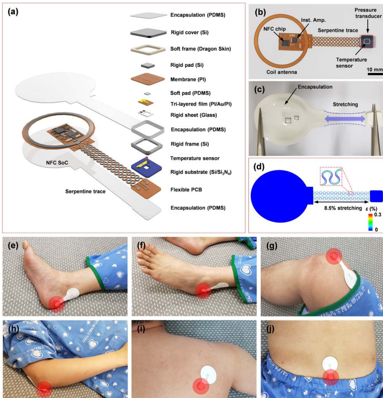
Fig. 1 Schematic illustrations and images of a battery-free, wireless pressure, and temperature-sensing platform. a Exploded view schematic illustration of the battery-free, wireless pressure and temperature-sensing platform. b Photograph of a device before packaging. c, d Photograph and FEA results for a packaged device in a stretched configuration. e–j Photographs of devices mounted on body locations that are susceptible to pressure injuries, including the heel, malleolus, knee, elbow, scapulae, and sacrum.
