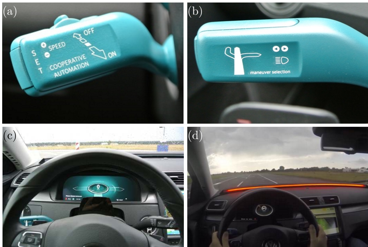
Figure 7.5: PRORETA 3 HMI components. Mode selection lever (a), maneuver selection lever (b), instrument cluster with driver monitoring camera (c), LED stripes (d).
