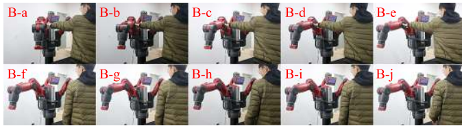
(b) the experimental results of impedance control with human motion intention estimation: seen from B-a to B-e, a human partner operates the robot to the target position 1; seen from B-f to B-j, the interaction torque disappears and the robot still remains in the current position.
