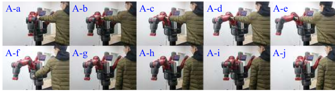
(a) the experimental results of impedance control without estimation: seen from A-a to A-e, a human partner operates the robot to the target position 1; seen from A-f to A-j, the interaction torque disappears and the robot moves back to the initial position.
