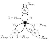
Figure 1: HMM model for 3 speakers with 1 state per speaker, with a dummy non-emitting (initial) state.
