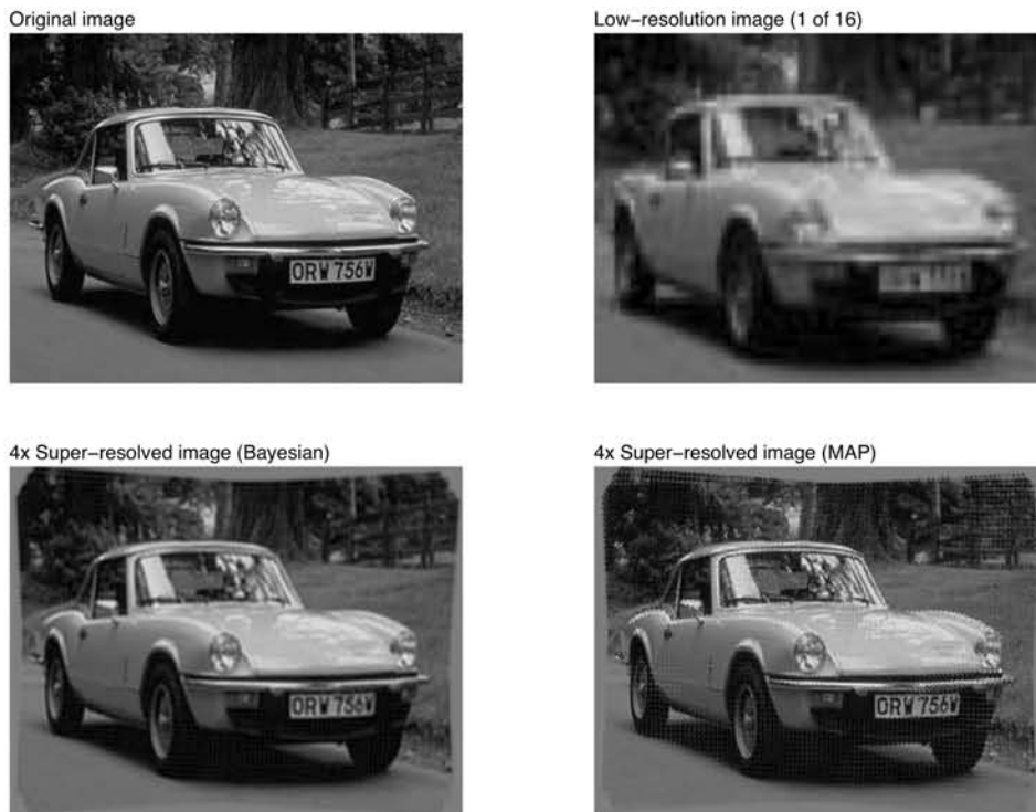
Figure 1: Example using synthetically generated data showing ( top left ) the original image, ( top right ) an example low resolution image and ( bottom left ) the inferred super-resolved image. Also shown, in ( bottom right ), is a comparison super-resolved image obtained by joint optimization with respect to the super-resolved image and the parameters, demonstrating the significantly poorer result.
