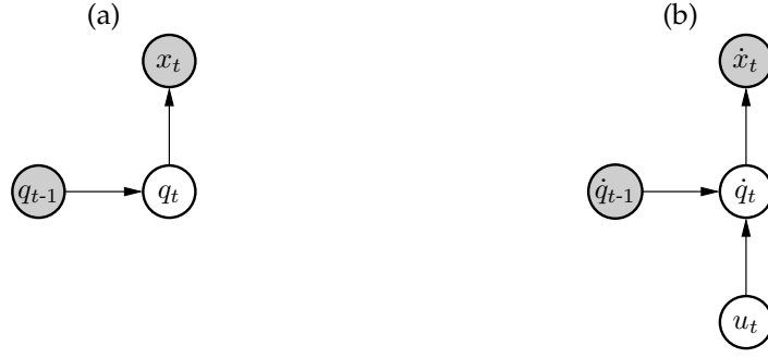
Figure 1: Graphical models of Bayesian control, (a) for motion rate control, (b) for dynamic control.
